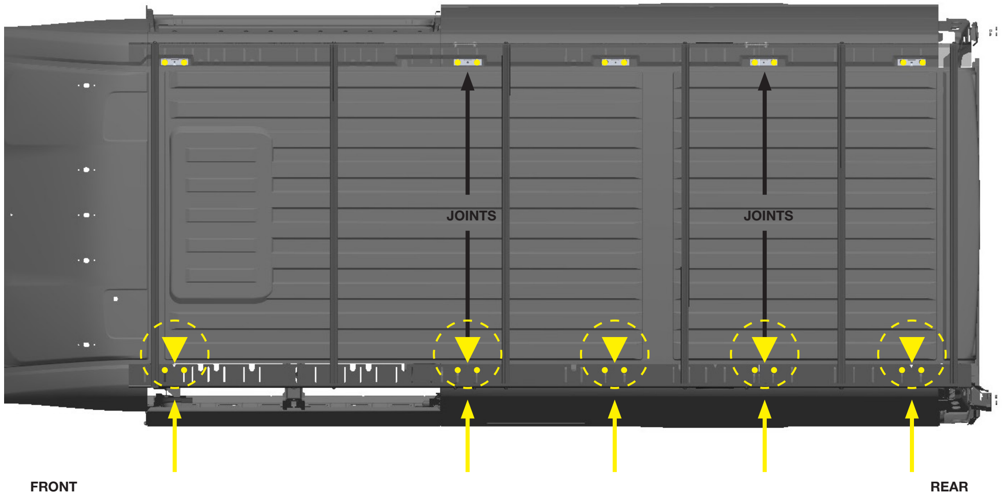
Side plate positioning diagram - RAM Promaster 159-X HR
